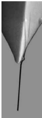
Carbon Nanotube STM Tip
